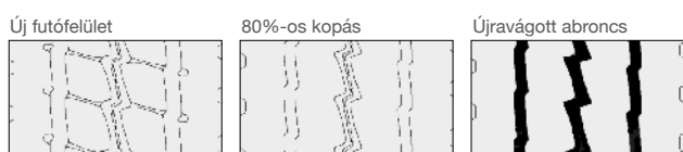
Maximum regrooving depth = 3 mm, regrooving width = 8 mm.
